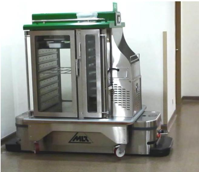
**Figure15: Typical AGV with a supply trolley**
